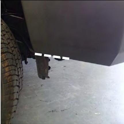
30. Trim inner wheel arch liner hanging below the bar. Trim horizontally inwards from the underside of the bulbar wing.
