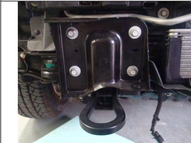
6. Once the bumper is off, remove the original bumper brackets from the chassis, and retain the bolts.
