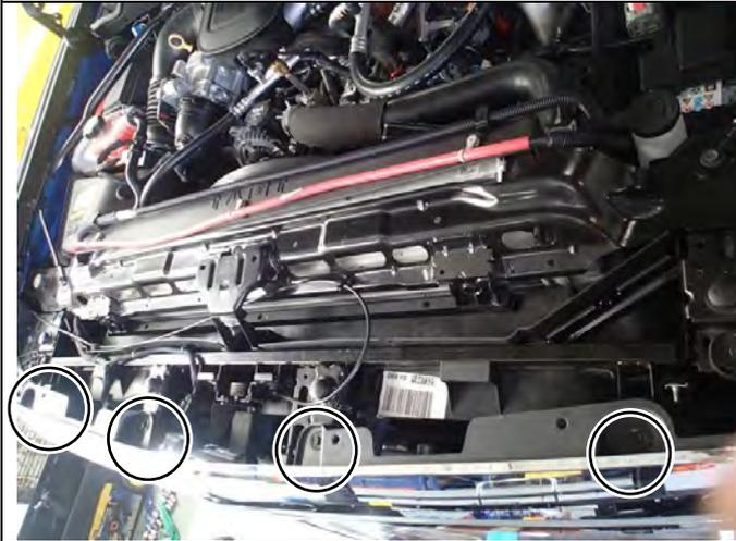
1. Remove engine bay cover to expose top of grille as shown.
