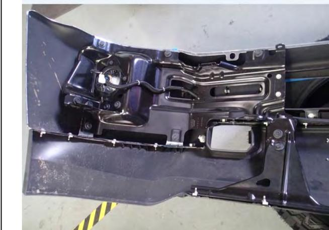
7. Remove the reinforcing from behind the OE bumper. Remove the original wiring loom and park sensors. Remove park sensors by spreading tabs apart and sliding sensors out the back face of the bar.
