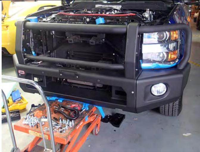
Tape is used under the headlights and under the bar to protect these areas from scratches during fitment.
