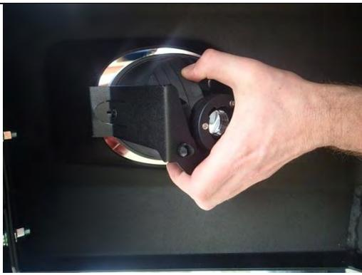
15. Remove globe from fog light by twisting anti clockwise.
