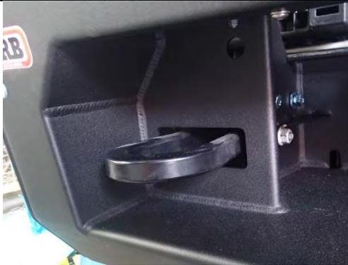
23. Fit tow hooks and reinforcing brackets into the bar
