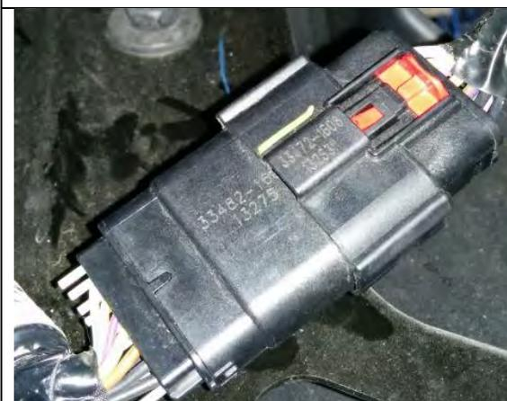
4. Underneath the bar, unbolt the wing braces and unplug the loom.
