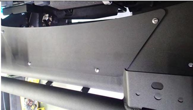
28. If no winch was fitted, fit the winch cover panel to the upper pan.
