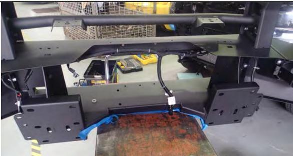
14. Fit parking sensors and loom to the bar as shown, ensure the original order of parking sensors is maintained. Route the loom across the back of the upper pan of the bar.
